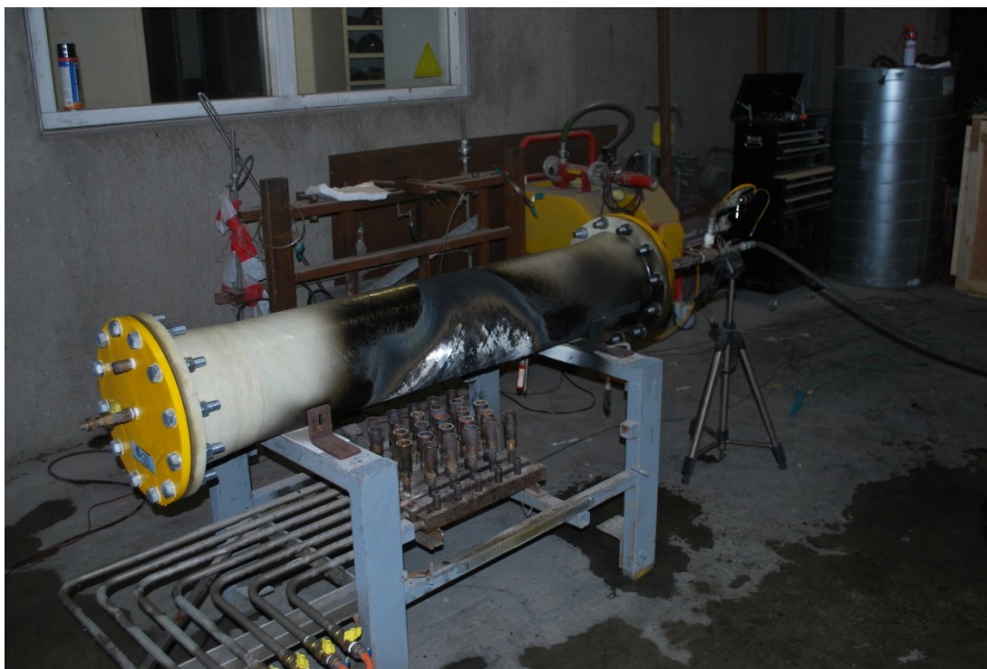
Figure D3 Specimen during the hydrostatic pressure test
